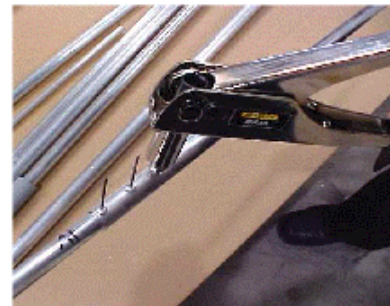
4) Slide rivet tool over mandrel and pull ("pop") the rivet
