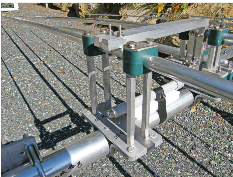
Figure 3 — The feed line connects to the balun near the center of the boom.
