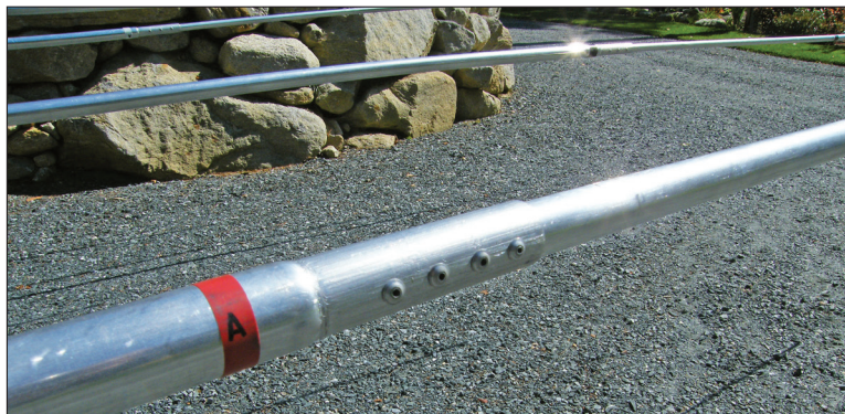
Figure 1 — Element joints use rivets to secure the sections. Element sections are well-marked with colored tape and labels.
