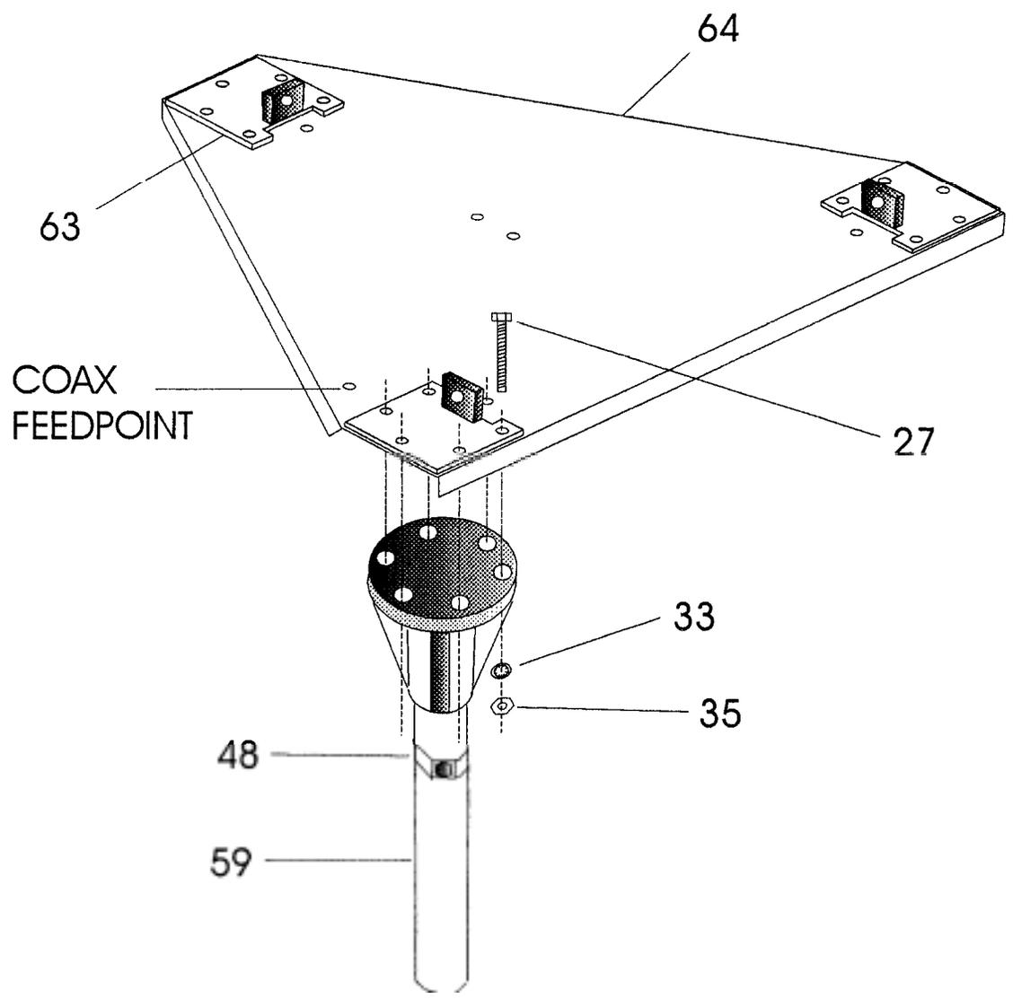
The tower plates inside the Hy-tower have been improved. The new plates are made from stainless steel, Install the lower plate as shown in the diagram, One X has been left out of the top section to allow for easy installment of the lower ( larger) triangle. Install two spacers between the triangle tab and the tower leg,
