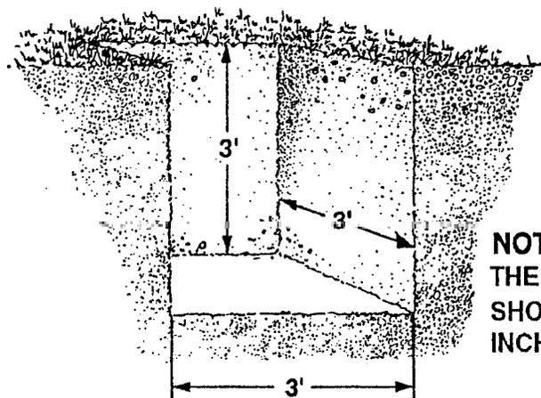
**NOTE: IN COLD CLIMATES THE DEPTH OF THE HOLE SHOULD BE A MINIMUM OF 6 INCHES BELOW FROST LINE**
