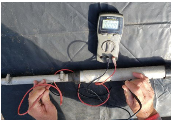
7 Measuring R between trap shield and element - should be <1 ohm
