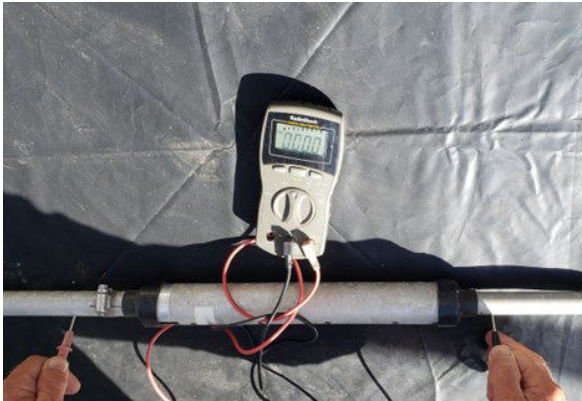
6 Measuring R across the trap - should be <1 ohm
