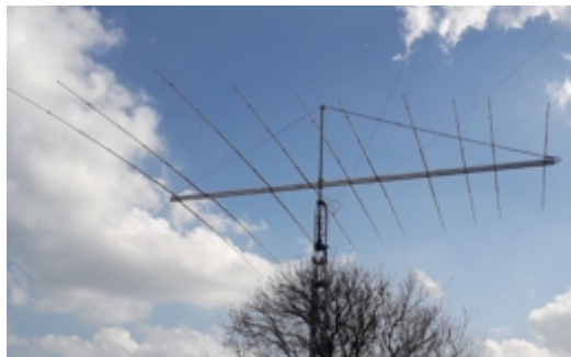
A BOLPA-10 with coax routed back along the forward guy
