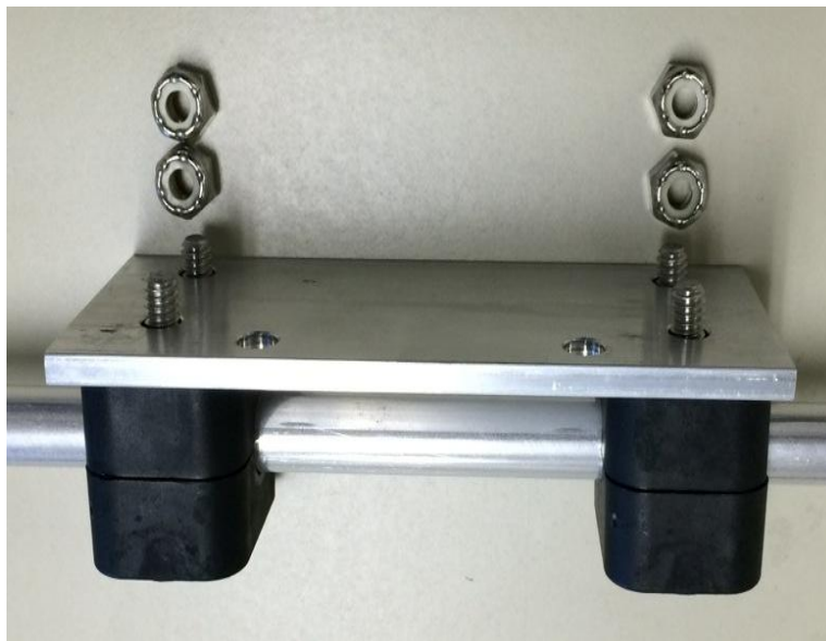
Element being mounted to Element Plate using Black Clamps and nylon nuts
