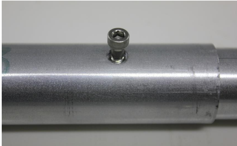
Screw fits into recessed hole – face up
