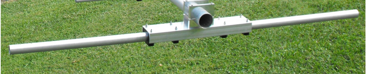
40M center sections mounted to boom using two (2) clamp sets
