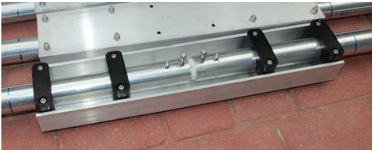
40M center sections mounted on element channels
