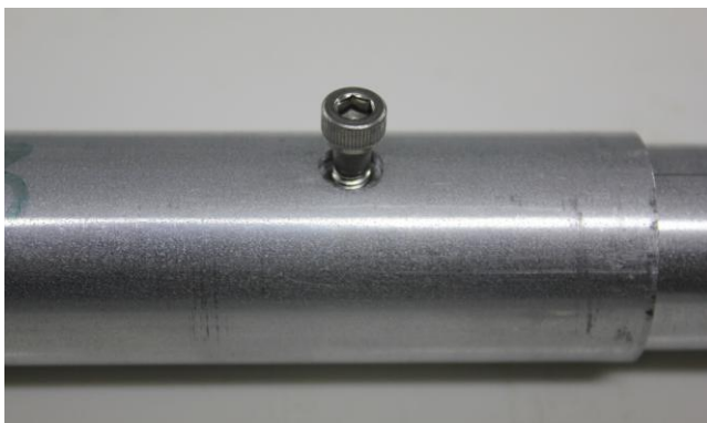
Screw fits into recessed hole - face up
