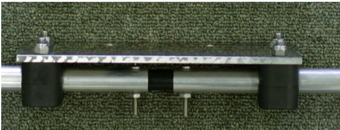
Completed Driven Element Assembly mounted on Element Plate
