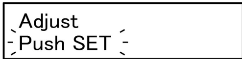
Figure 28: Adjust [Push SET] is blinking. Press ⓂSET to see an AEU name blink. Press ⓂSET to determine what AEU to check.
