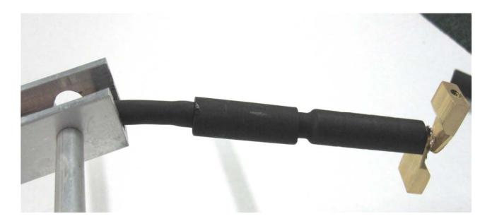
5. Carefully slide the cable and feed nose assembly back into the boom assembly, align the grounded side of the feed nose assembly with the hole in the front of the boom assembly and add the 8-32 x 3/8 screw.
