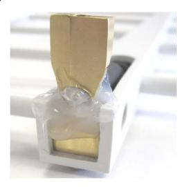
6. Add silicone sealant or equivalent around the feed nose and solder connections as to seal for long term installation. Use appropriate topography sealing techniques for long term installation.
