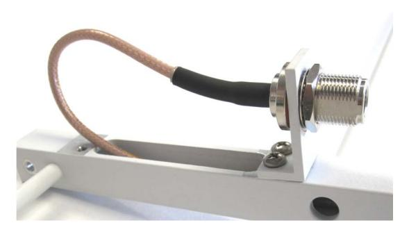
5. Route the N connector thru the connector mount bracket, add lock washer and nut and tighten.
