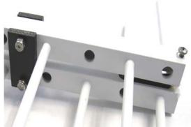
8. Locate the BTM side plate, BTM block and mast mount plate. See the picture and assemble the BTM bracket. Add the u-bolts and uni-cradles for your mounting style, horizontal or vertical polarity. Be sure to tighten all hardware before installation. Always use good low loss coax for feed line. Seal all exposed connectors with the appropriate sealing techniques for your particular topography.
