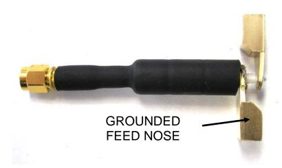
4.Slide on the supplied 1/2 shrink tube onto the cable. Attach the feed nose assembly to the end of the cable, slide the shrink tube over the mating SMA connectors and shrink.
