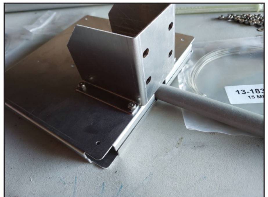
Photo F. Mounting box (for the mast) and the coax feed tube that will be used for the matchbox and coax attachment.
