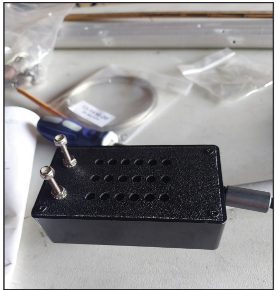
Photo H. Matchbox holes for the MFJ 1836H (the H stands for high power) to vent out heat and moisture. It is important to have the holes facing towards the ground.
