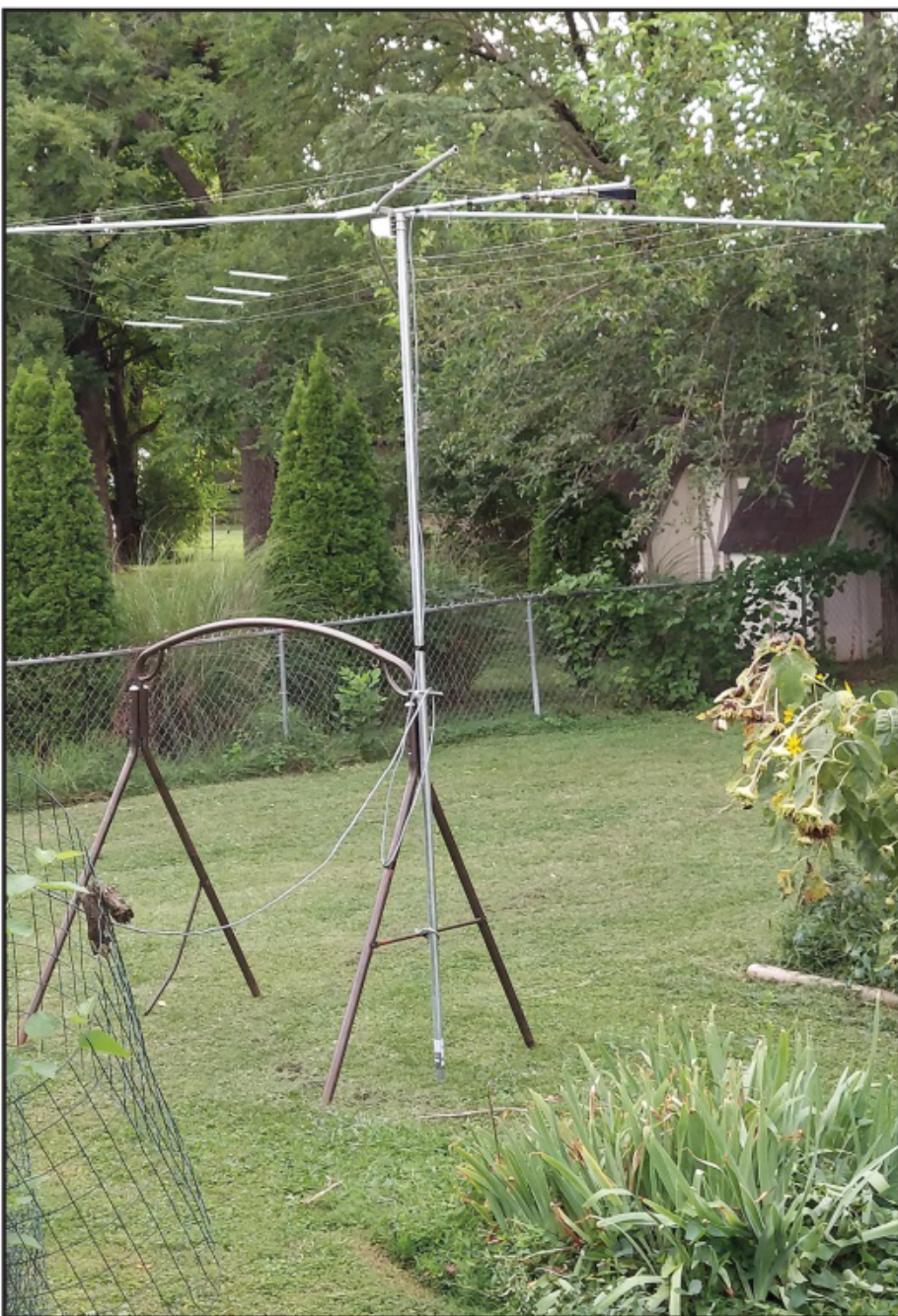
Photo K. Completed cobweb antenna, up 10 feet on a chain-link fence top rail.
