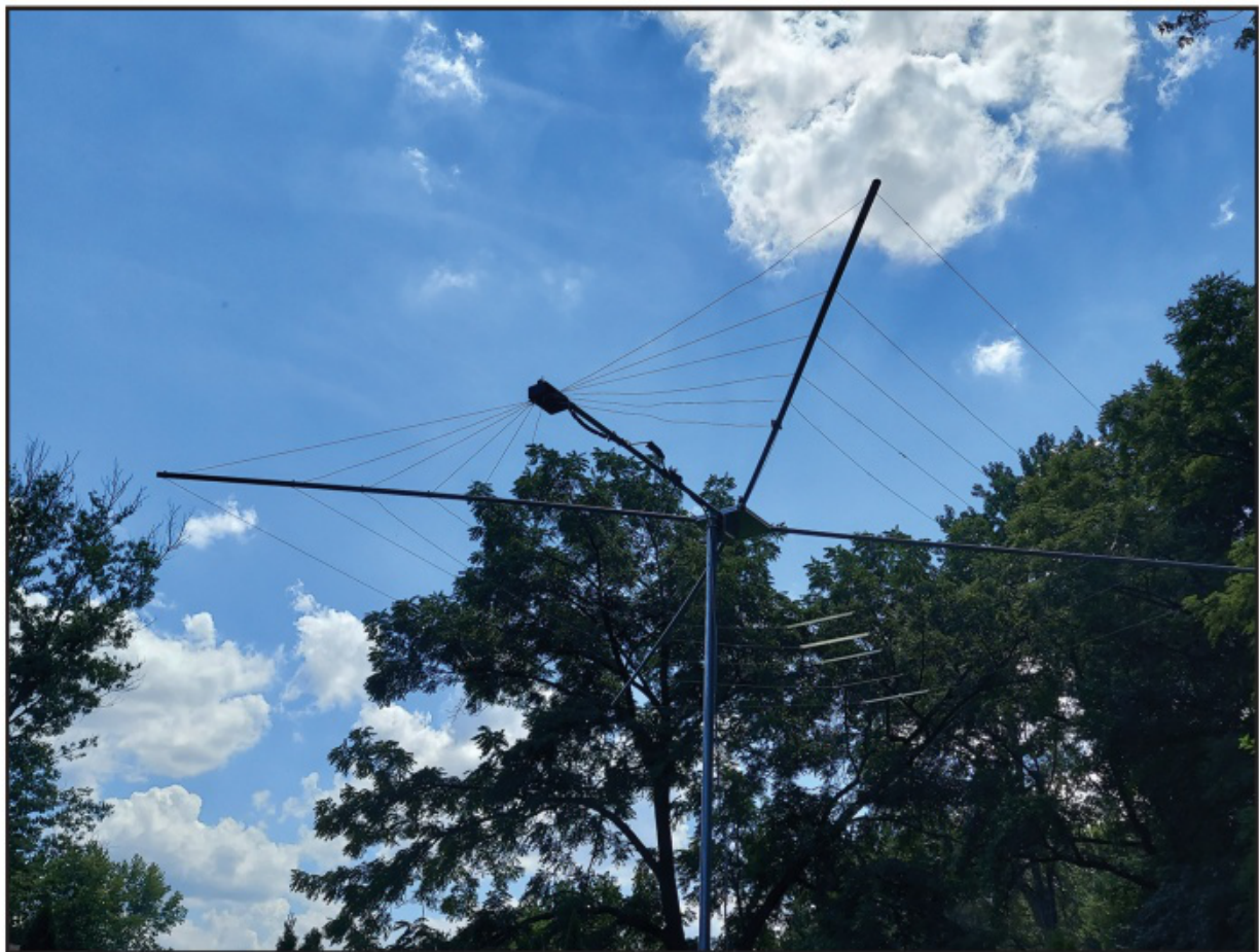
Photo J. Upward view of the cobweb silhouetted against the blue sky makes it easy to see the matchbox wire element feed point and the terminated wire elements insulator strips.
