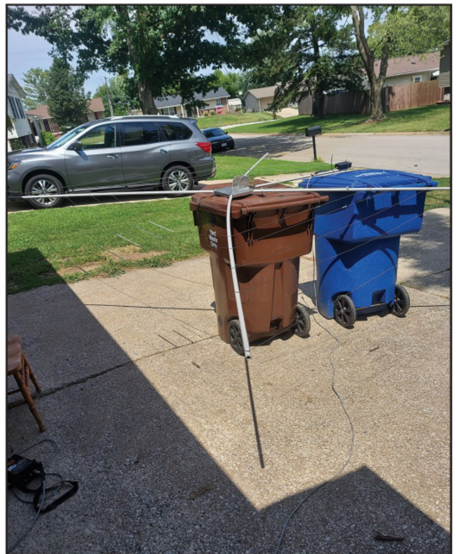
Photo I. MFJ recommends elevating the cobweb to 6 feet for pruning the antenna for optimum SWR. I used my nonconductive trash cans to hold my cobweb up for tuning. It wasn’t off the ground six feet, but I took that into account while shortening the wire elements.
