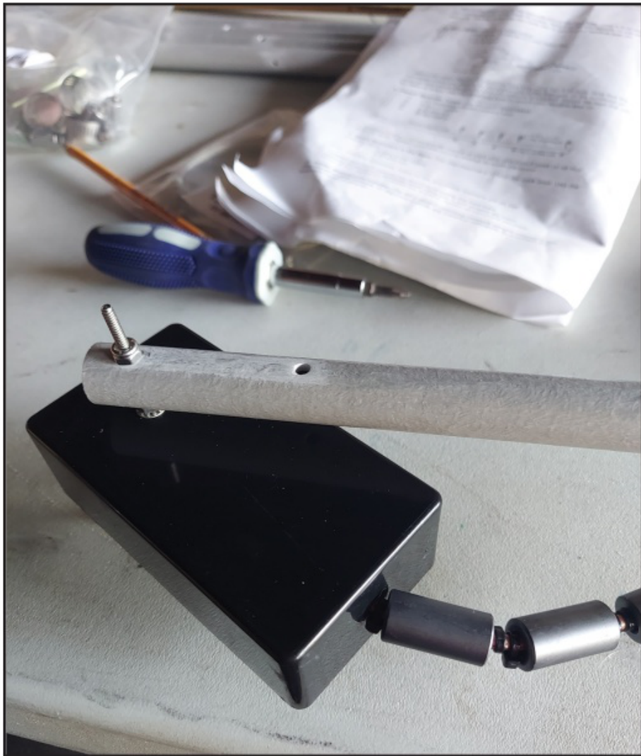
Photo G. MFJ 1836H Matchbox, UHF coax jack (SO-239) and ferrite beads to reduce RF current flow on the outside of the coax.
