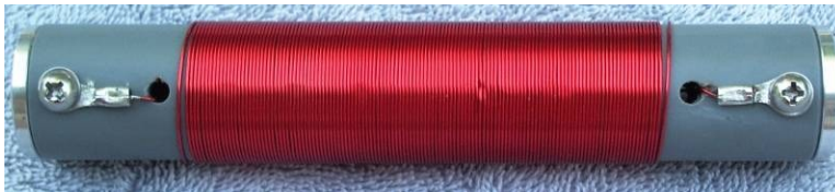
The Completed 80 meter coil
