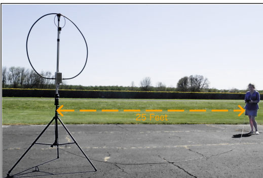
Fig. 9 Recommended 25 foot distance
