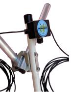
Note: The support assembly from steps i - iii does not need to be taken apart to use the antenna in another location. It can be transported as a complete unit.
