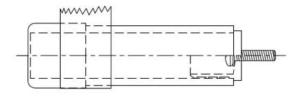
[ ] Mark places for the holes in a straight line as shown below and drill Ø5/64" holes thru to the inside only. The 11/16" location will go thru the copper and PEX tubing, the 2 3/4" location thru the PEX tubing and PEX brass plug..
