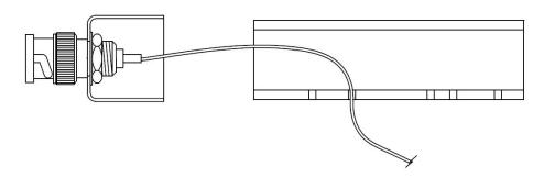
[ ] Slide the PEX tubing into the copper pipe plug until the two 11/16" location holes align, and secure the two with one of the 4-40 x .25" screws.
