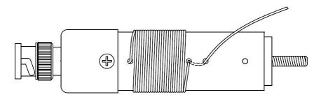
[ ] The 22awg wire needs to be connected to the PEX plug. Remove the enamel insulation from the wire where the wire wraps around the screw and secure the 4-40 screw as shown below.
