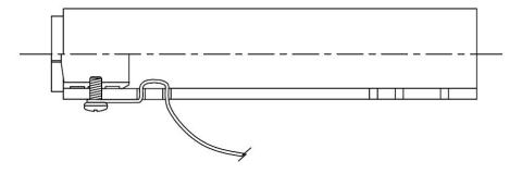
[ ] Wind a total of **61 turns** close wound, and feed the far end of the magnet wire down thru the hole location shown to the inside, and back to the outside thru the next hole. You can now trim, leaving 3" of the 22awg magnet wire. Re-install the PEX, making sure the 4-40 hole lings up.
