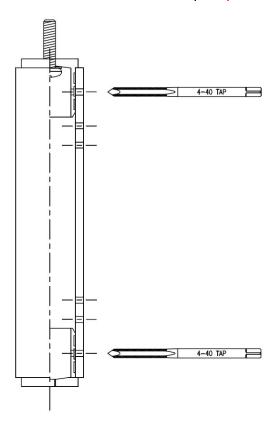
[ ] Remove the PEX plug with the screw assembly attached and set aside. Thread one end of the #22awg magnet wire into the hole shown, and back out the other hole shown. The 22 awg wire needs to be connected to the PEX plug. Remove the enamel insulation from the wire where the wire wraps around the screw and secure the 4-40 screw as shown below.
