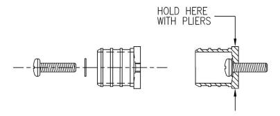
[ ] Slide the piece of PEX tubing into the copper pipe plug all the way to the bottom and tape with scotch tape to prevent it from rotating. Place the PEX plug from the operation above into the open end of the PEX pipe.
