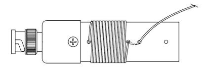
[ ] Press the PEX plug/screw assembly back into the open end of the PEX tubing all the way to the shoulder of the plug and line up the 4-40 tapped holes.
