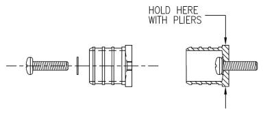
Press both PEX plugs into the 4" length of PEX pipe. Measure and mark the PEX pipe as shown below, and drill the six holes Ø5/64", thru to the inside only.
