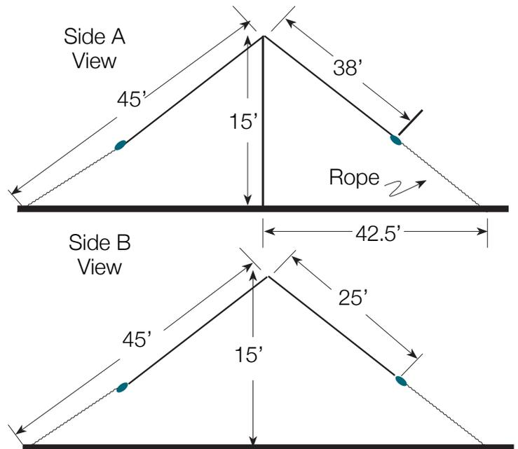
The EZ NVIS is ready to deploy NVIS antenna based on an article by Carl Jelnick, N6VNG (SK). He based his design on the AS-2259/GR a military, dual band NVIS antenna set. The antenna comes with a center support and the four assembled and marked antenna elements. You need to add rope, coax and an appropriate mast. The antenna is constructed from 14ga Soft Drawn copper wire.
