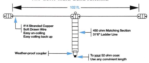
This antenna should be supported with rope or other nonconductor.
