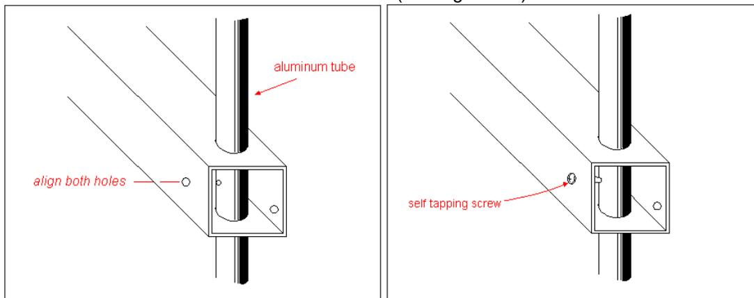
**Figure 6.7** Inserting the aluminum tube into the mounting channel.
