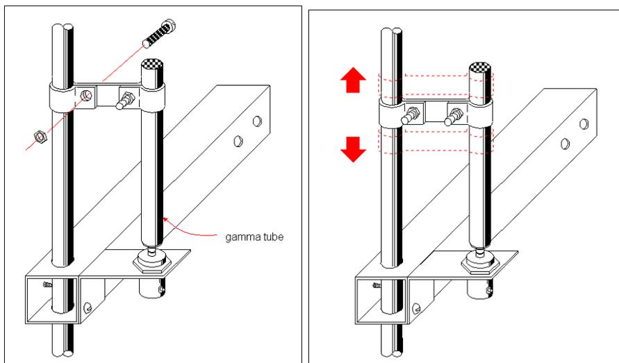
**Figure 6.10** Assembling the gamma tube into the gamma match.
