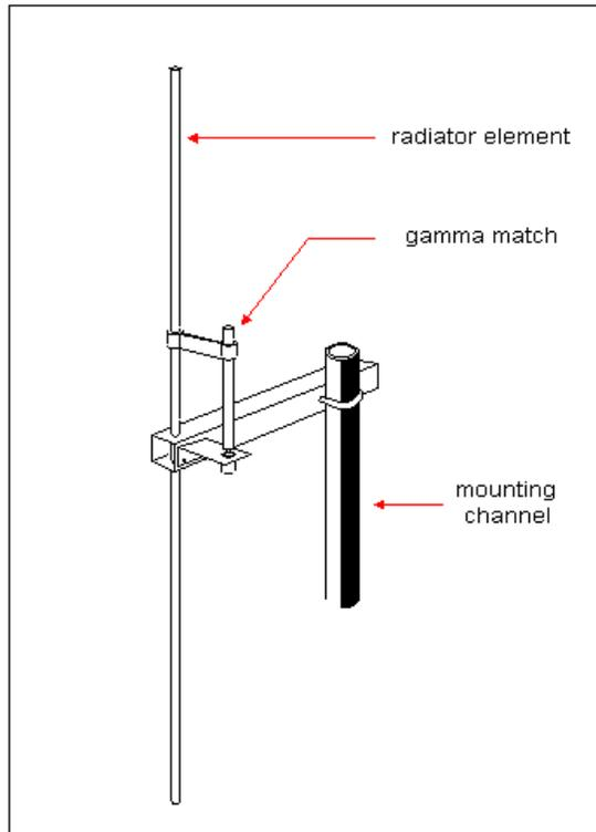
Insert the aluminum tube through the large hole and align the hole at its middle part to the 1/8" diameter hole at the side of the channel (see Figure 6.7).
