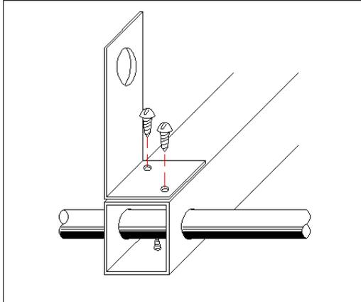
**Figure 6.9** Fixing the feedpoint bracket on the mounting channel.
