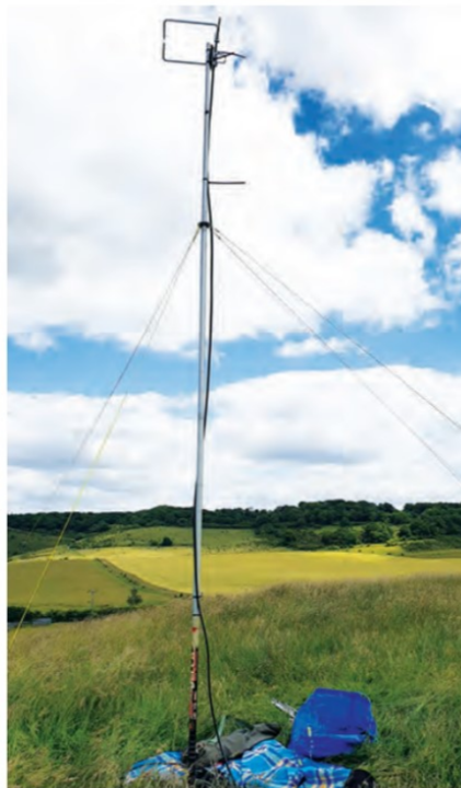
The Sharman HLP-270 Halo on the mast while testing it during the second RSGB 2m Backpackers Contest.
