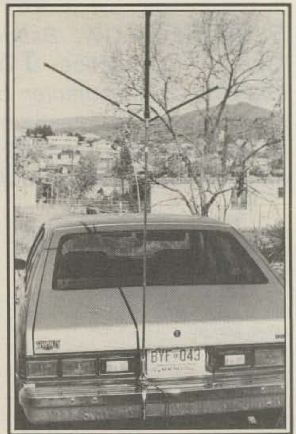
The Spider Antenna is shown in two installations. On the left it is mounted on the rear of the author's RV, and on the right it is bumper-mounted to his car.
