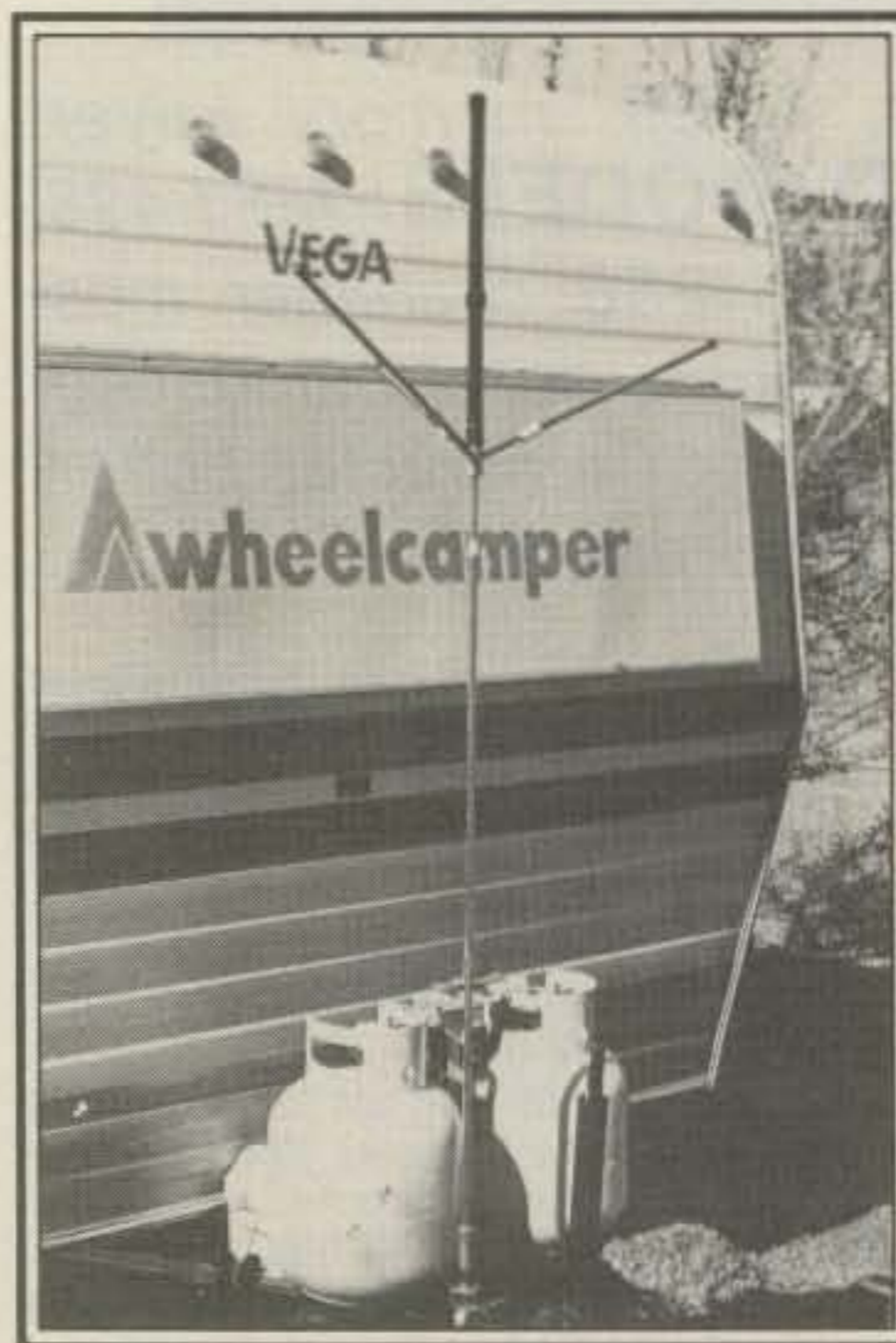
The Spider Antenna is shown in two installations. On the left it is mounted on the rear of the author's RV, and on the right it is bumper-mounted to his car.
