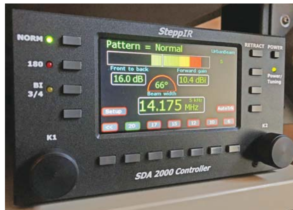
Figure 7 — The optional SDA 2000 controller offers many additional features compared to the standard SDA 100.
