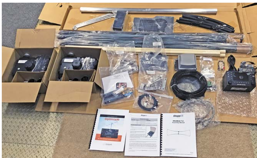
Figure 6 — All the parts that came with the author's UrbanBeam kit.
