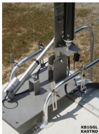
Picture 4 – MT-1 & Automatic Lift & Lay
