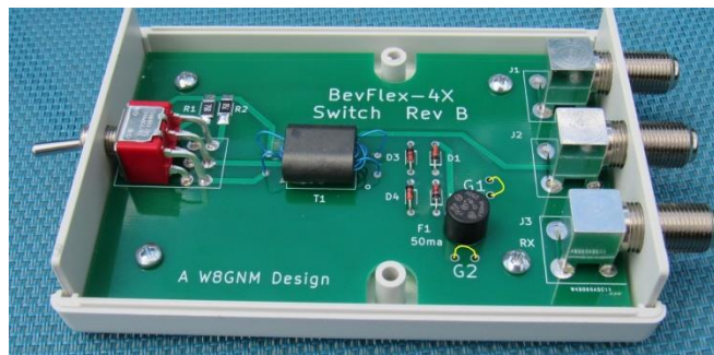
Figure 1. The yellow lines show installation points of optional jumpers.
