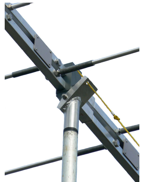
Pivot adjustment mount to alter between horizontal and vertical polarisation. Can be secured in either polarisation with the included rope.
