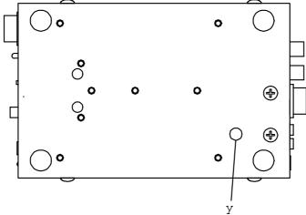
y. Microphone output (Radio Input) level (Refer to setting level adjustment on page 13 for details)
