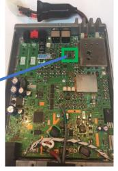
When removing C1473 use either a dual SMT tip on a temperature-controlled soldering station or two temperature-controlled irons with small (1/16 inch) tips. It is important to melt the solder on both ends
