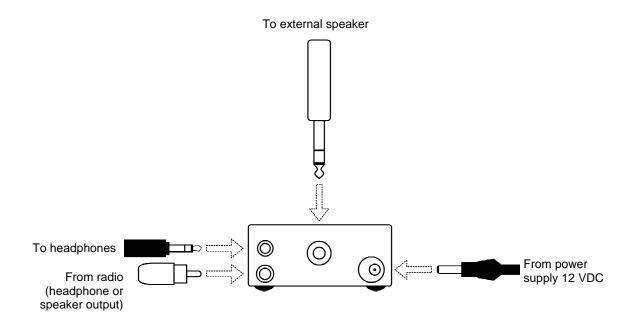
By default, the large phone jack (1/4", 6.35 mm) is set up for the external speaker, and the small phone jack (3.5 mm, 1/8") is set up for headphones. If desired, the large phone jack can be set up for headphones and the small phone jack for the external speaker; see page 2.
