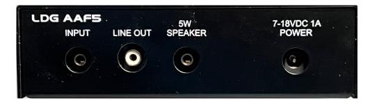
**Input:** Audio input jack, 3.5 mm (1/8") stereo tip-ring-sleeve jack
