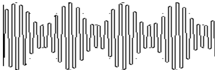
Figure 6 — A carrier signal with modulation
