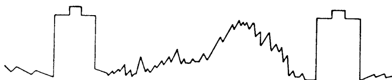
Figure 4 Normal Video and Sync Signal.
