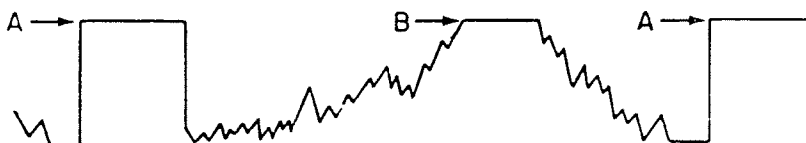
Figure 5 Overloaded or Clipped Video and Sync Signal.
