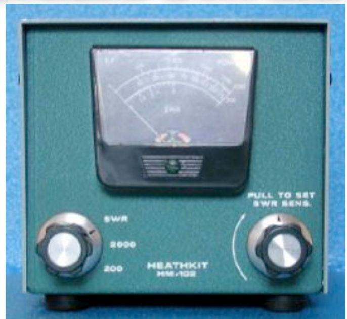
Fig 1: Heathkit HM-102 HF RF Power Meter. The HM-2102 Meter for VHF is Similar.
