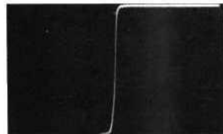
FIG. 6. Rise time of the square wave section of the IG-18. Distance between graticule divisions = 0.1 \mu sec. The author says the tiny ring at the top is test lead inductance.
