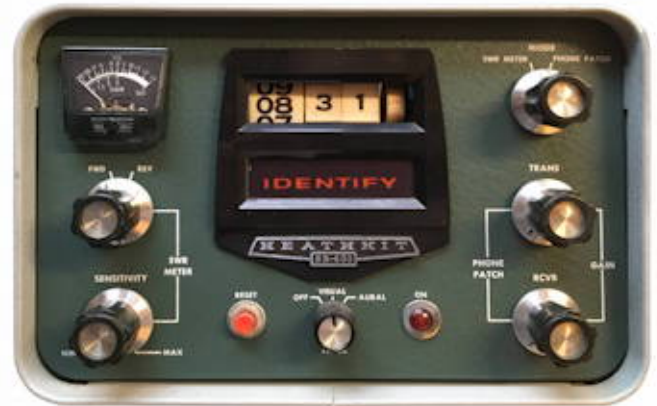
Figure 1: Heathkit SB-630 Station Console combines clock, phone patch, SWR bridge and 10 minute timer into one package.
