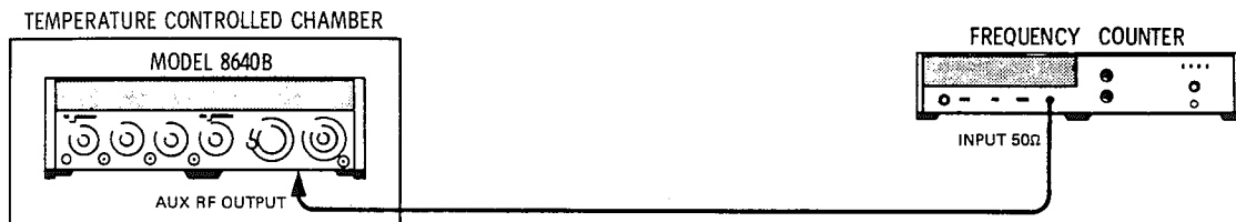
Figure 4-2. Frequency stability vs Temperature Test Setup
