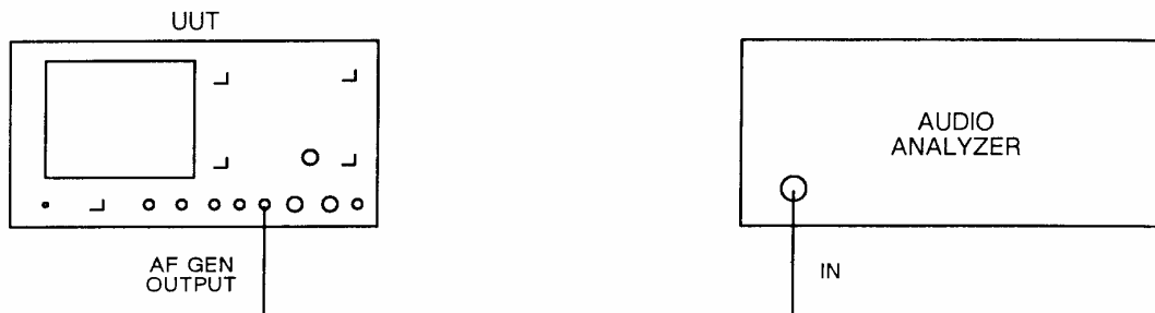
Fig 5-16 Test equipment connections for AF generator residual noise spurious signals performance checks
