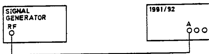
Figure 6.33 - Connections for Minimum Time Interval PVP
