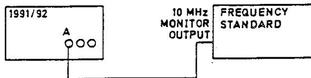
Figure 6.26 - Connections for Internal Frequency Standard Adjustment
