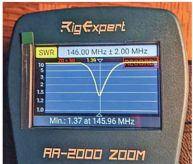
Figure 1 — SWR sweep of a 2-meter band-pass filter observed on the AA-2000 ZOOM screen.
