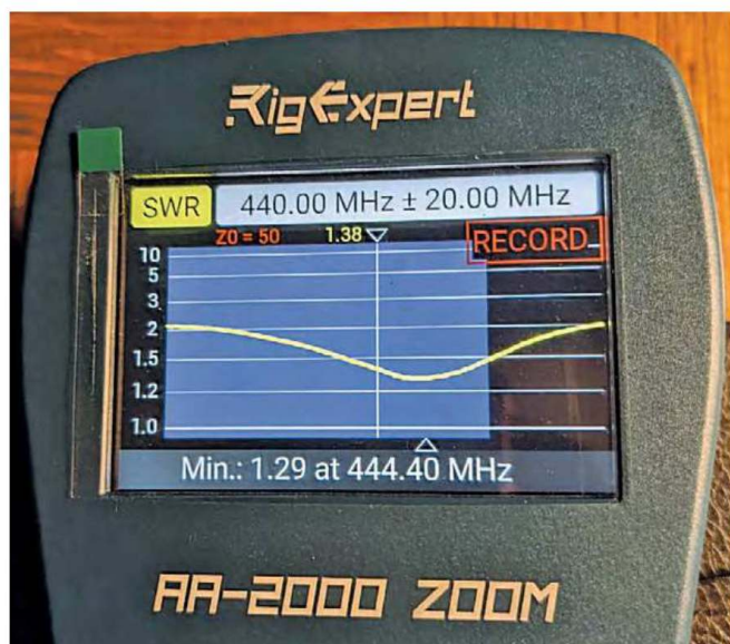
Figure 3 — SWR sweep of a 440 MHz mobile antenna observed on the AA-2000 ZOOM screen.
