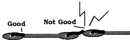
**“Solder”** When you are directed to *solder*, this means to solder the part’s leads in place, and to inspect both (or all) solder connections for flaws or solder bridges. If no soldering problems are noted, nip off the excess protruding leads with a sharp pair of side cutters.
