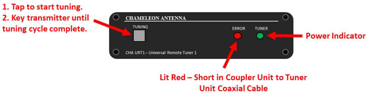
Figure 10. Coupler Unit Operation.
