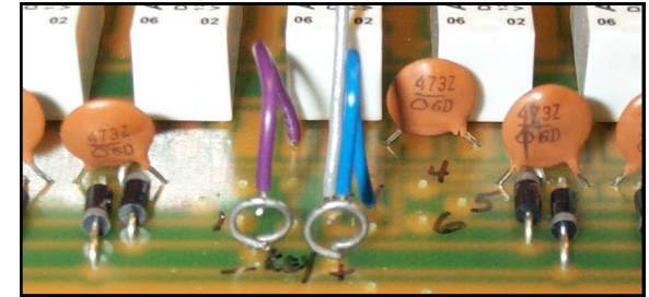
Jumpered for Negative Keying
