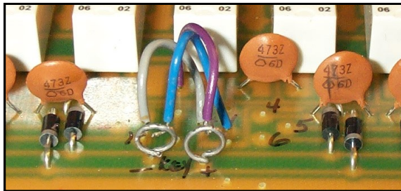
Jumpered for Positive Keying
