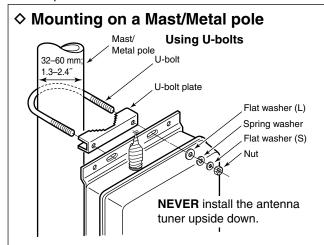
⚠ **WARNING!** Mount the AT-140 securely with the supplied nuts and bolts. Otherwise, vibrations and shocks due to waves could loosen the antenna tuner making if fall, causing personal injury.
