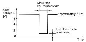
\*For the Tuner Through function; Less than 250 milliseconds
