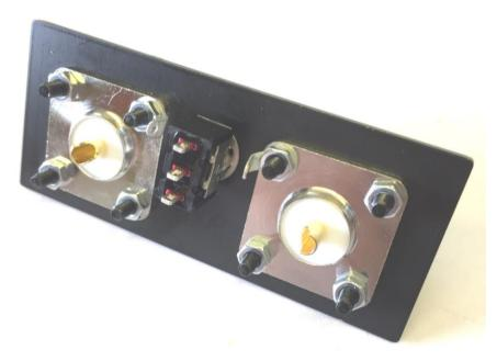
Use the screws/nuts provided to mount the sockets to the back panel. Place the two earth tags on the back of the socket on the holes nearest the switch as per the picture here. If using BNC's tighten the sockets and make sure the earth tag is on the side near the switch.
