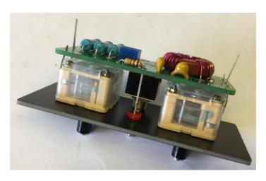
Carefully make sure that the three legs of each capacitor go into their correct mounting holes and that the LED isn't trapped or falls out while doing this. A bit fiddly I know.
