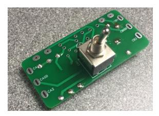
Now turn the board over so we can fit the switch, remove the top nut and washers from the switch and put them on one side for later. The switch should be fitted so its pins **JUST** fit flush with the other side of the PCB, this is so when the ATU is assembled into the case and onto the front plate there is enough of the screws thread protruding to attach the nut to. The nut is only cosmetic really so fitting it really is optional.
