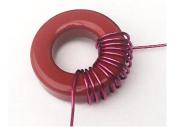
the one end about 50mm long. This counts as one turn, every time the wire passes through the core it counts as a turn,
