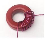
Continue to wind the wire for a total of 13 turns as in the picture on the right.
