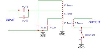
13/6/13 turns on the primary and 7 turns on the secondary, the output can be isolated by means of a grounded toggle switch so the user can use either balance or unbalanced antennas.
