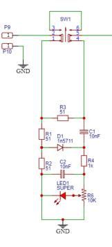
This section can be switched IN or OUT by a two way toggle switch, when in circuit the bridge will light the LED if the antenna is presenting an impedance higher (or Lower) than 50 ohms, if the impedance is matched the LED will go out. Depending on the power level in use the LED can be either too bright and doesn't go out when matched or to dim and hard to see. This circuit has an adjustable sensitive trimmer and it is best to adjust this to suit your most likely used power level.
