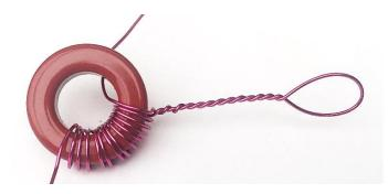
Form a loop about 30-50mm long as shown here, feed the wire back into the core and wind for another 6 turns.
