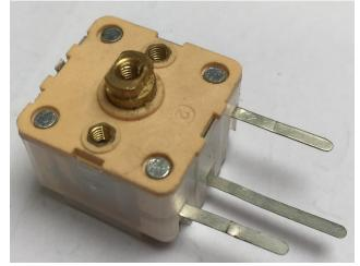
If you have a suitable capacitance meter check between the center pin and the two outer pins, you should find that you have about 250-270pf when you adjust the capacitor between each pin and center.
