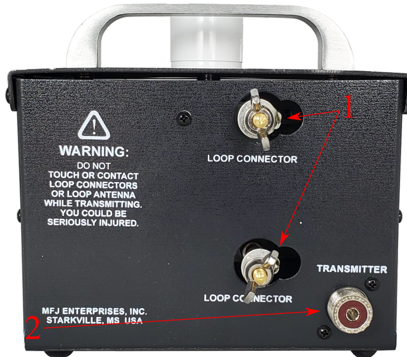
Figure 5: Rear-panel Connections: 1.) Wire loop connectors, 2.) Coax input
