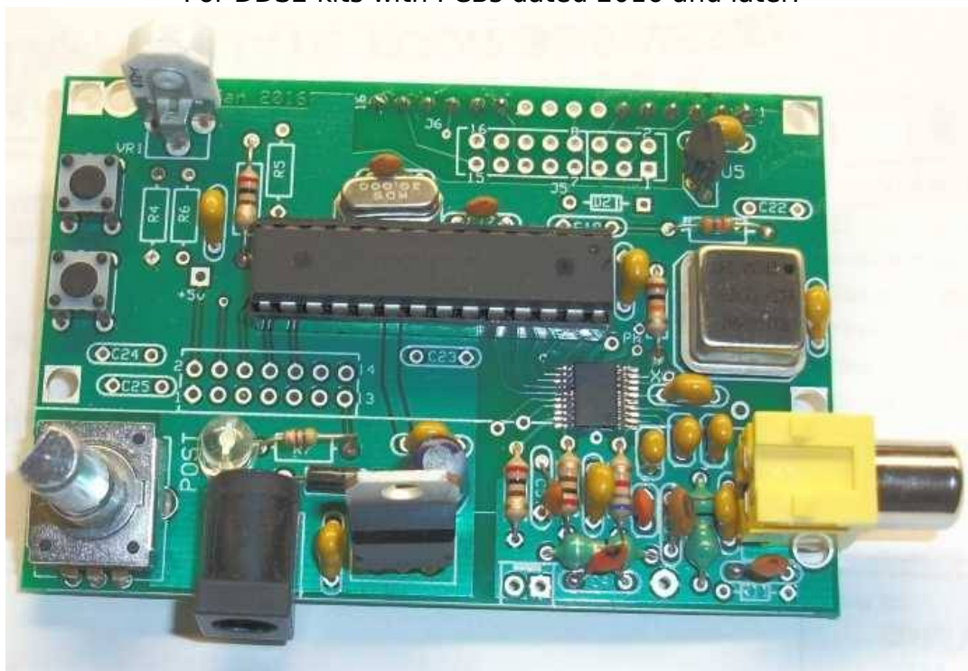
The above photo is of the Jan 2016 PCB, Later PCBs have different mounting holes and the Output jack was turned 90 degrees. Identical electrical schematic though.
