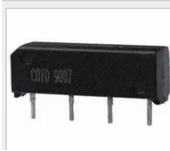
Figure 1-4. Reed Relay. Device is symmetrical, center pins are the coil, end pins are the contacts.
