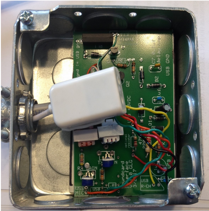
Figure 3-3. Printed circuit board mounted (actually wedged) into a 4" electrical box. One knockout has been removed to allow access to the potentiometers, The USB dongle is also inserted, and another knockout has been removed and a "3/8 non-metallic clamp" used to secure the wires' exit point. There is a standard solid metal plate that fits on top as a cover.
