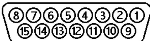
DSUB-15 Male wiring side
