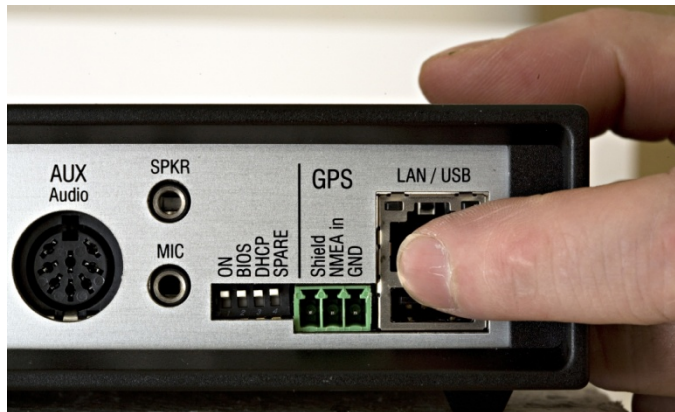
Figure 4: Pushing out the mainboard
