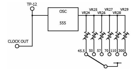
The baud rate clock adjusts the voltage applied to pin 7 of timer IC, and necessary frequencies are picked up.
