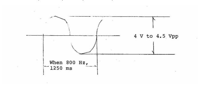
If malfunction often occurs due to noise, vary the resistance of R28. When the resistance is increased, malfunction by noise decreases, whereas the sensitivity drops.
