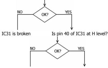
R76 is broken; C32 is shorted; trouble of RESET switch or switch wiring; breakage of IC27, IC18, IC2, IC32, IC31
