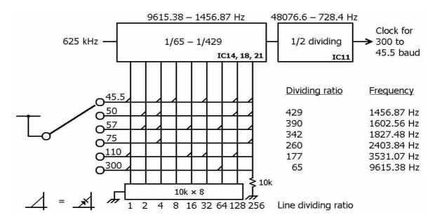
The dividing output of IC14, 18, 21 is the total of dividing ratios in all lines. The output being divided by this divider is divided again to 1/2 and converted to a necessary frequency of 50 % duty to delivered. This output of baud rate clock can be checked on the TP-10.
