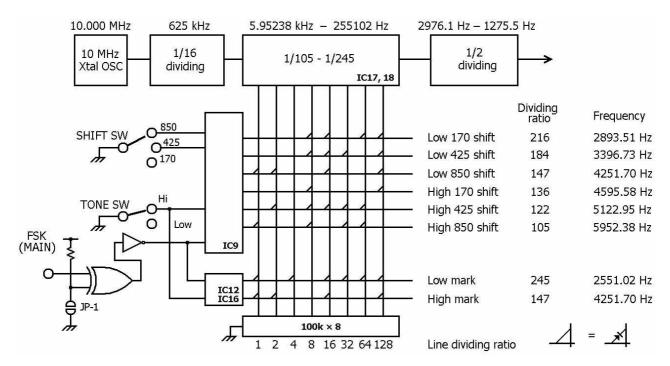
The dividing output of IC17, 18 is the total of dividing ratios in all lines where diodes are provided,
