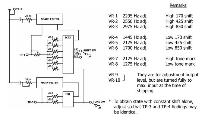
The selected frequency can be checked on TP-3 and TP-4. Part of this output is amplified by the LED amplifier, and is used to light up the LEDs of mark and space. Also signals for X, Y oscilloscope of the monitor are taken out from this output.
